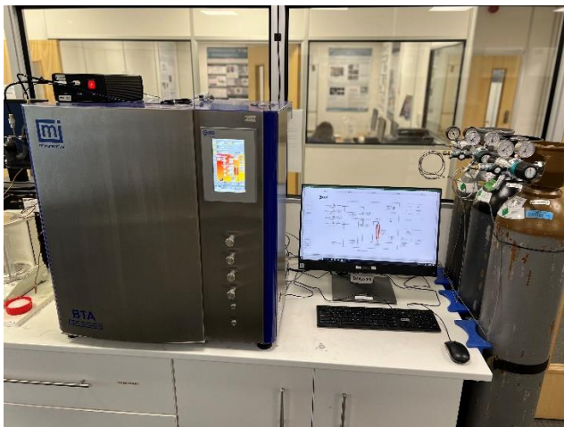
Figure 6: Promethean's new state of the art break-through analyser (BTA) (left) and resultant break-through curves for a representative MOF exposed to simulated flue gas at three different adsorption temperatures (right). These curves show how no CO 2 is being detected downstream of the BTA's MOF bed for different periods of time. The MOF eventually becomes saturated and post-MOF CO 2 "breakthrough" is then detected.
